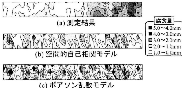
Fig.7 腐食量等高線図 (CR-350-3)
