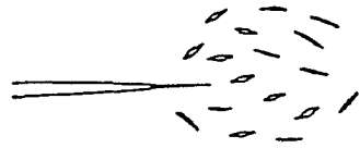
Fig. 7. Main crack-microcracks interaction model
