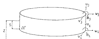
Fig. 2 Finite element (shell)
