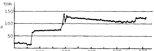
Fig. 11 Variation of the Load Range with Cycles
