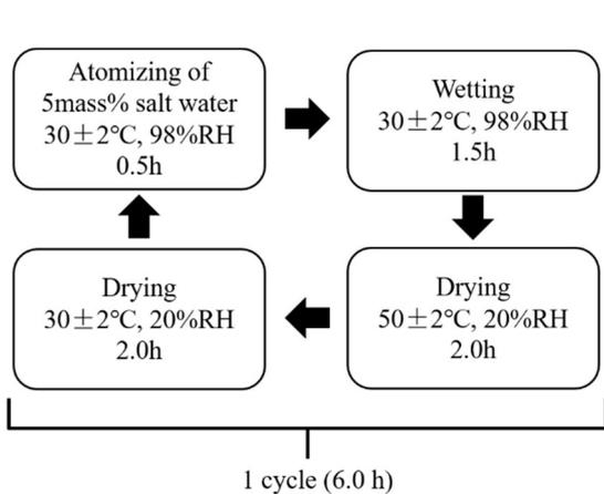
Fig. 1 Corrosion cycle applied during the accelerated exposure tests
