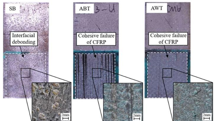
Fig.6 Failure surfaces after tensile tests
