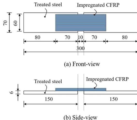
Fig. 2 Geometry of CFRP-steel single strapped joint (unit: mm)
