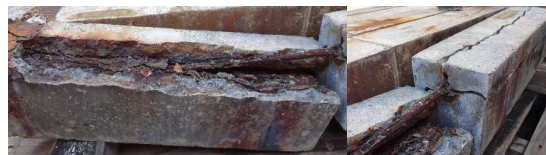
Figure2. Specimen with joint but no treatment condition (J1)
