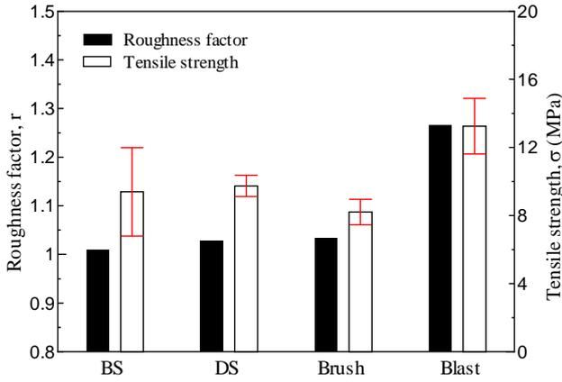
Fig.2 Roughness factor and adhesion strength of steel substrate
