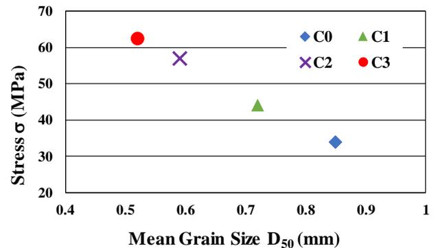
Fig. 2. Stress obtained from single particle strength test for crushed GBFS
