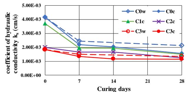
Fig. 4. Coefficient of hydraulic conductivity of crushed and aged GBFS
