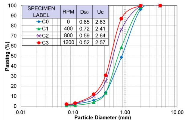
**Fig. 1.** The particle distribution curve of crushed GBFS
