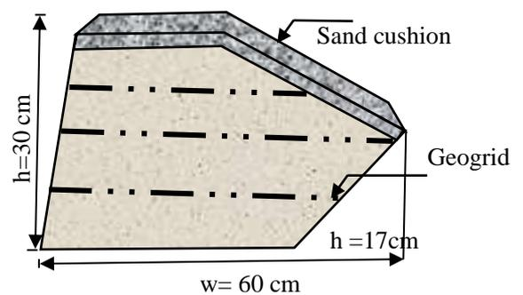
Fig2. Schematic embankment model
