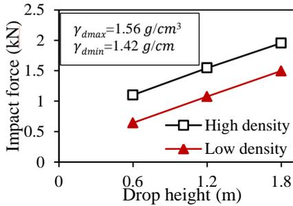
Fig3. Impact force with drop height and different density
