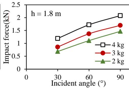
Fig4. Impact force drop height with Incident angle and different weights
