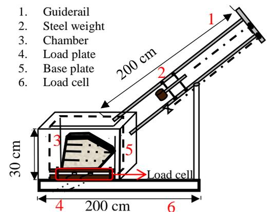
Fig1. Drop weight falling impact test
