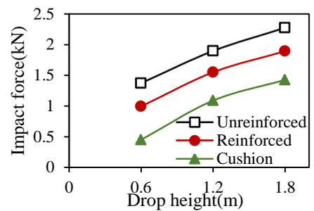
Fig 5. Impact force drop height for reinforced and cushion with different weight
