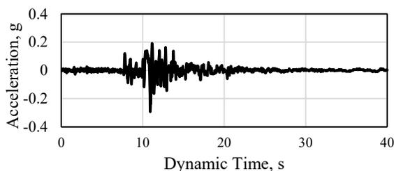
Figure 3. Seismic Input motion applied in the Analyses
