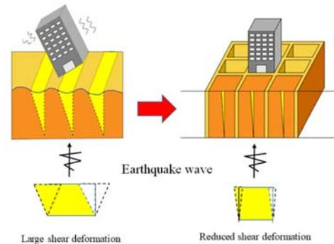
Figure 1. The mechanism of the grid-form deep cement mixing wall method
