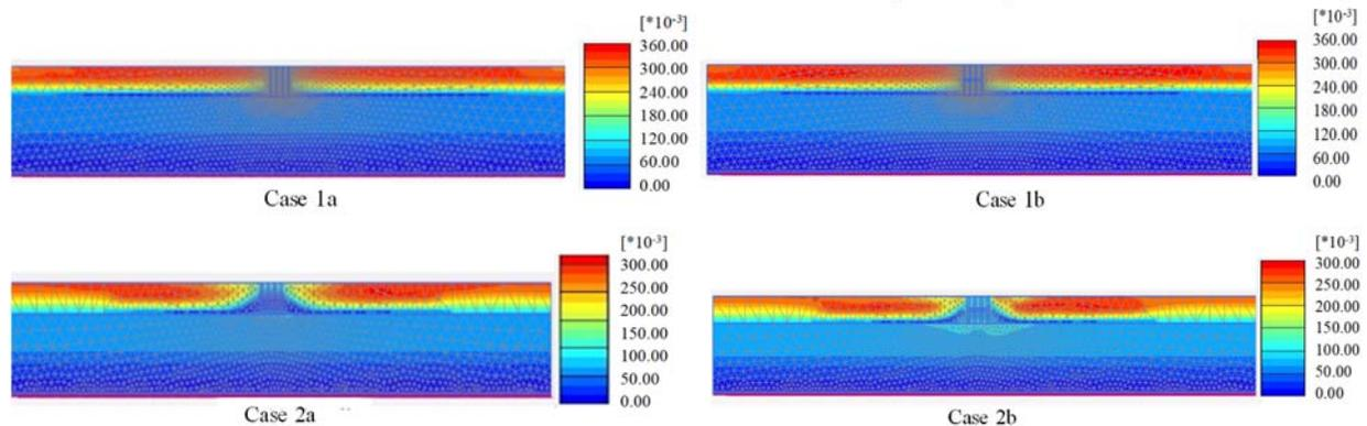
Figure 5. Total displacement due to the various ground improved cases at the end of the earthquake
