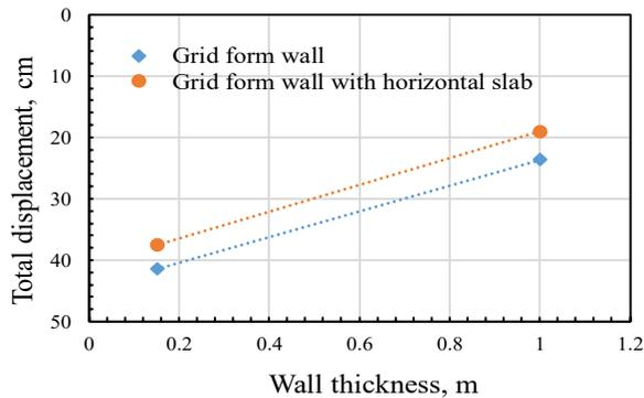
Figure 3. Maximum total displacements measured from different ground improved cases
