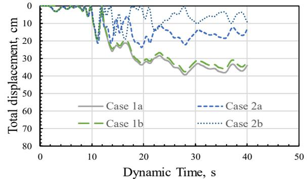
Figure 4. Time histories of the total displacement measured from different ground improved cases
