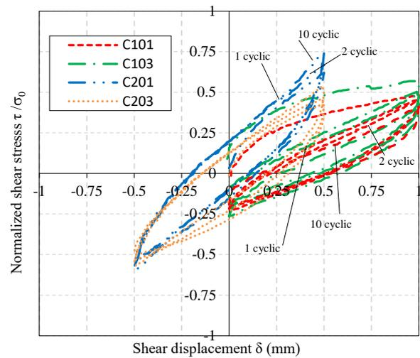
Fig. 3. Cyclic shear stress - displacement behaviour under one-sided and two-sided shearing for the overconsolidated area
