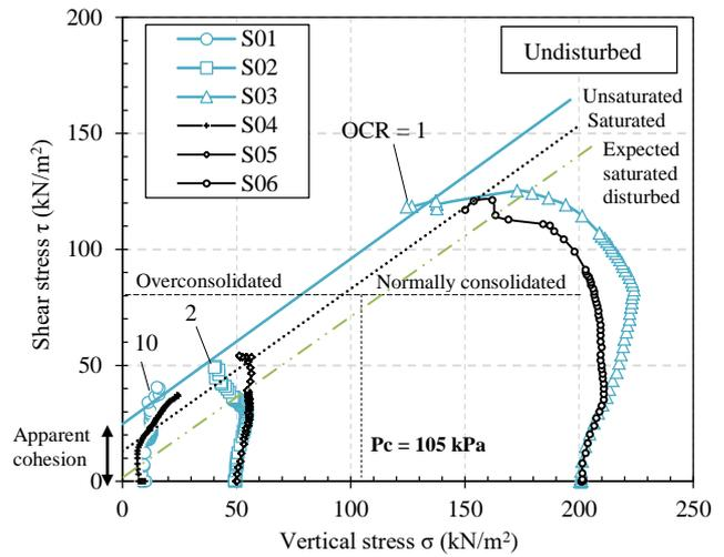
Fig. 2. Stress path static test unsaturated and saturated sample
