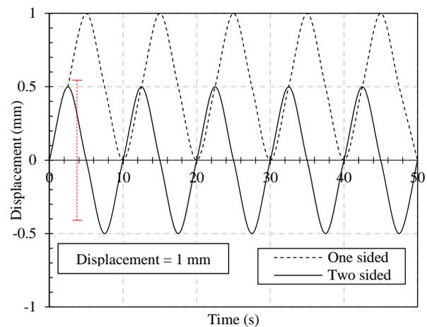
Fig. 1. Schematic of (one-sided and two-sided) cyclic loading.
