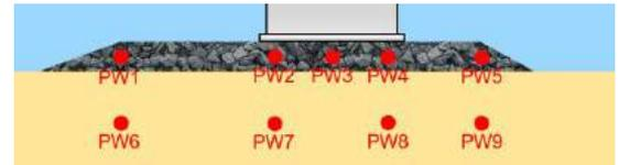
Fig. 7 Pore water pressure gauges
