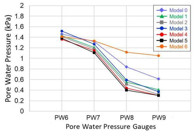
Fig. 9 Pore water pressure (in the foundation)
