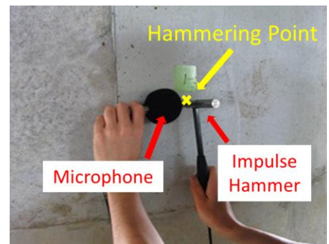
Photo 1 Impulse hammering test
