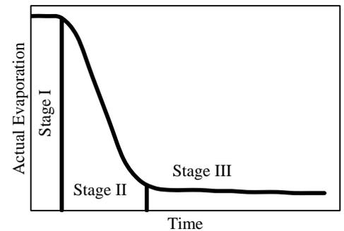
Fig.1. Actual evaporation stages. (Schematic).
