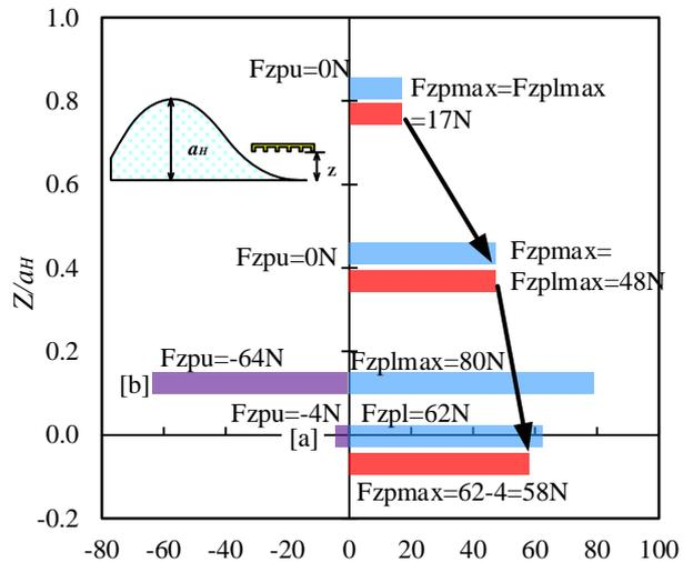
Fig. 7 Relationship between  $Z/a_H$  and vertical acting force
