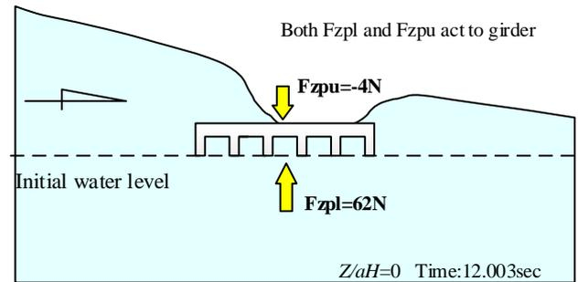
Fig. 6 Wave surface when  $F_z$  reaches peak ( $z/a_H = 0$ )
