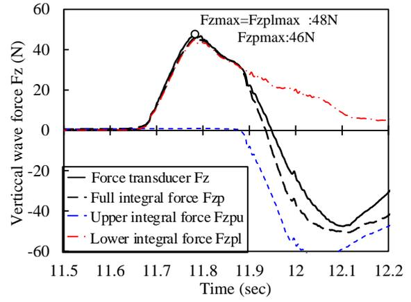
Fig. 4 Vertical acting force on girder model ( $z/a_H = 0.4$ )
