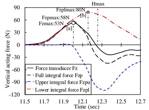
Fig. 5 Vertical acting force on girder model ( $z/a_H = 0$ )
