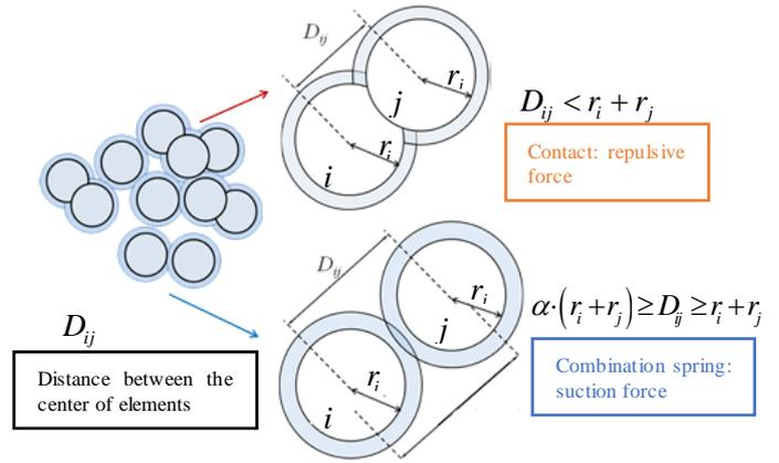
Fig.4 Modeling of suction effect by virtual water screen
