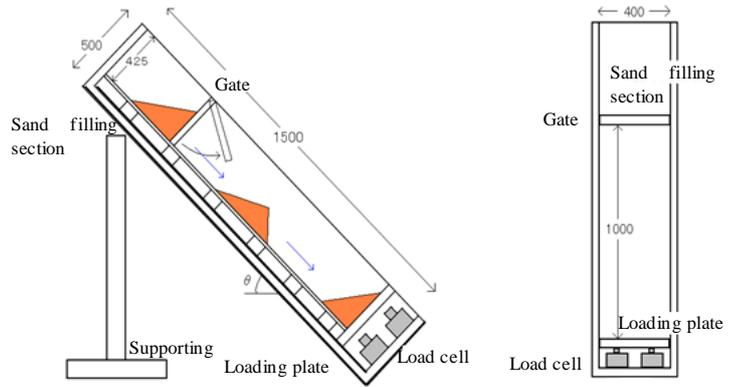
Fig.1 Setting of the model slope experiment (Unit: mm)
