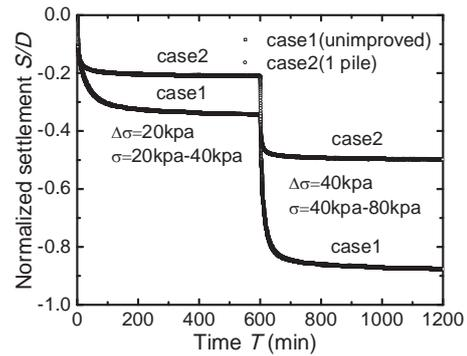
Fig. 3 Relationship between settlement and elapsed time
