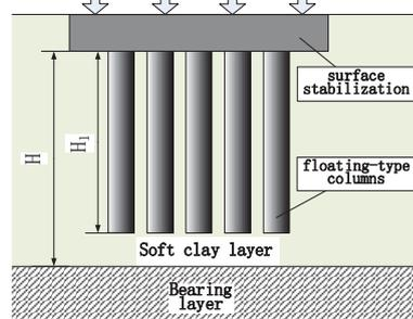
Fig. 1 Concept of floating type ground improvement
