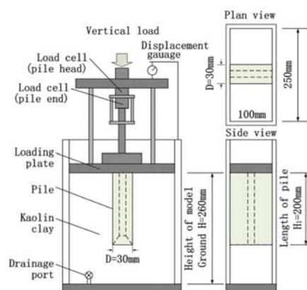
Fig. 2 Loading model test under the plane strain condition
