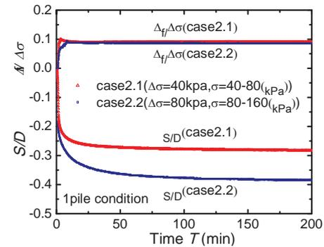
Fig. 4 Relationship between settlement, skin friction and elapsed time
