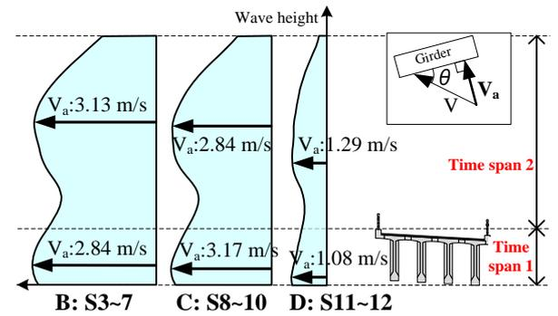
Fig. 5 Relationship between Wave Height and Velocity
