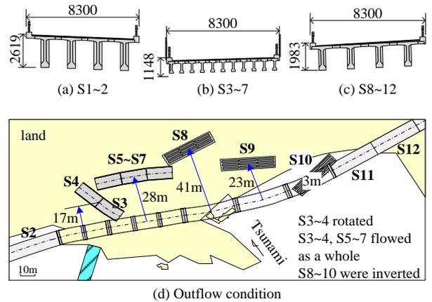
Fig. 1 Outflow Condition of Utatsu Bridge
