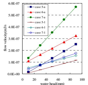
Fig.8 Flow velocity of fracture 1 in cross fractures
