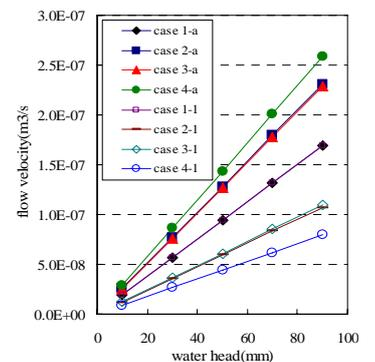
Fig.7 Flow velocity of fracture 1 in a single fracture
