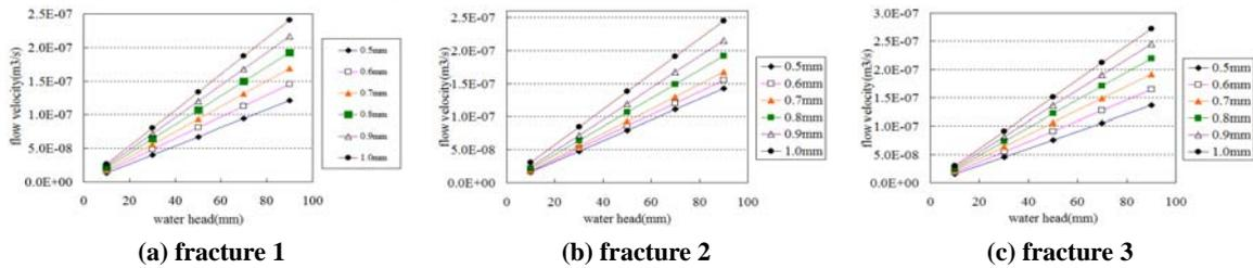
Fig. 5 Flow velocity under different apertures and water heads
