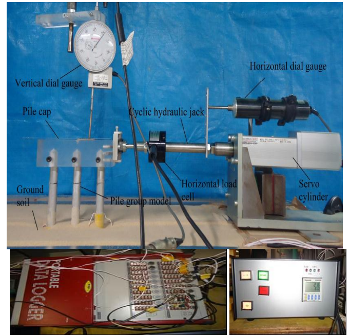
Figure 1 Horizontal cyclic loading system and measuring apparatus, data logger, and external control unit
