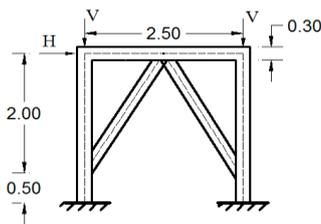
Fig. 1. Rigid frame with brace member
