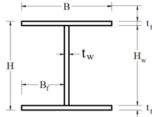
Fig. 4. I-beam section
