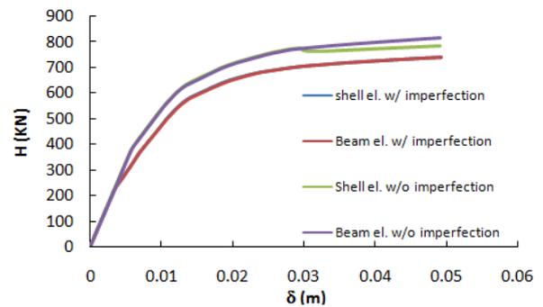
Fig. 6 Lateral load vs. lateral displacement curve of steel frame
