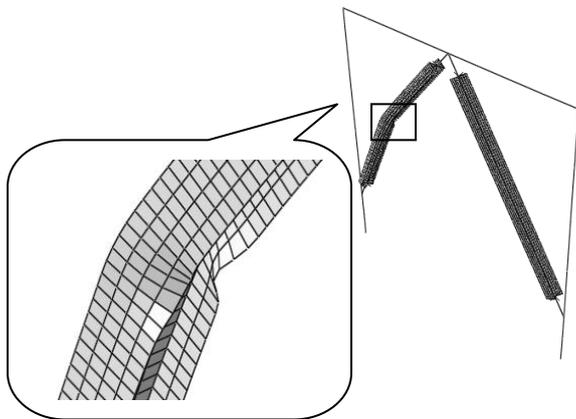
Fig. 5 Local buckling effect in case of imperfection
