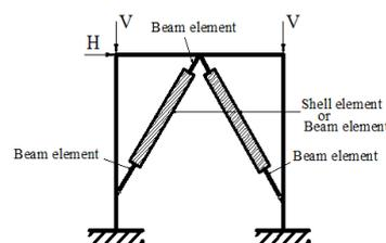
Fig. 2. Numerical model using shell and beam elements
