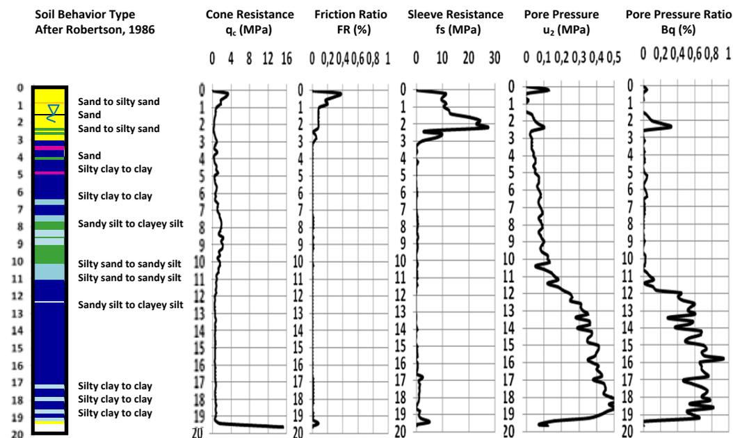
Figure 4. Test Result and geostatigraphy for CPTU-02
