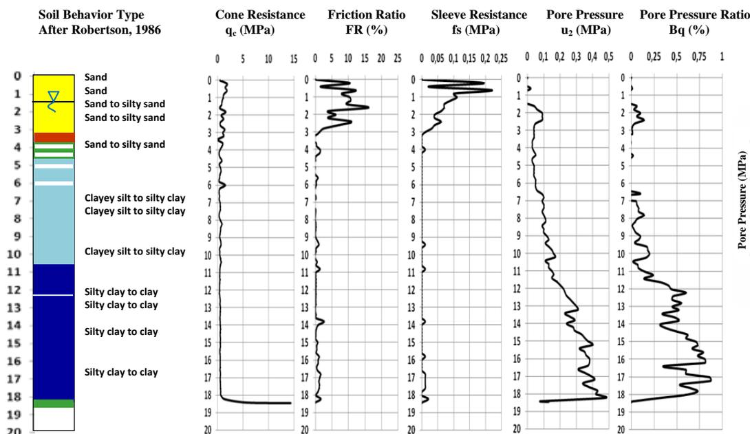
Figure 2. Test Result and geostatigraphy for CPTU-01
