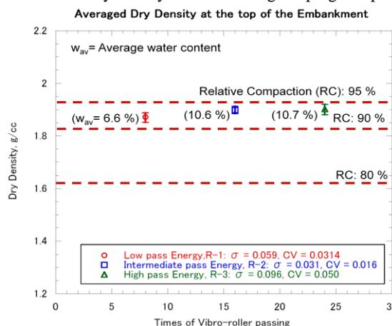
Fig. 4 Increase in dry density by vibro-roller compaction.
