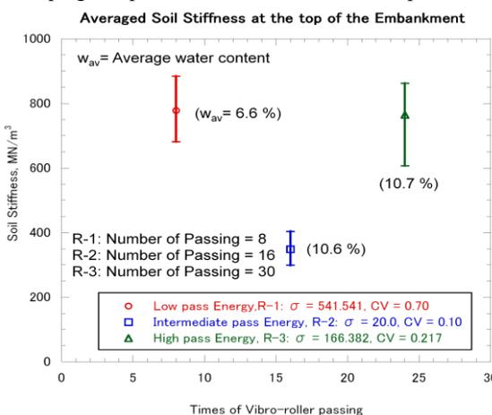
Fig. 6 Fluctuations of stiffness by vibro-roller compaction.
