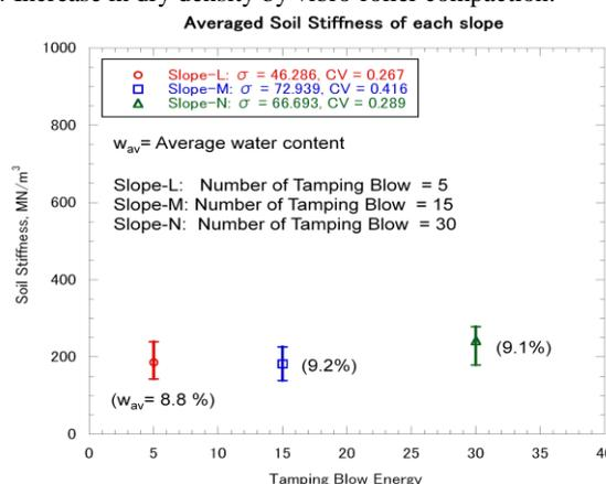
Fig. 5 Tamping compaction increases stiffness in slopes.
