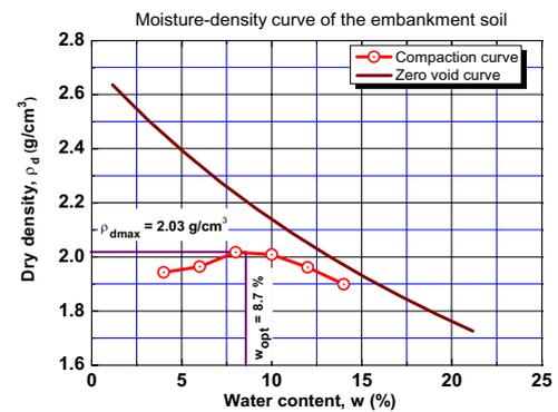
Fig. 2 Moisture density curve of the embankment soil.
