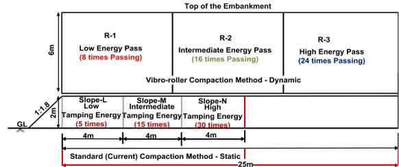
Fig. 1 Geometry of the construction of field embankment.
