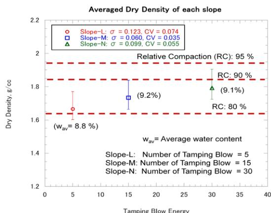
Fig. 3 Increase of dry density with increasing tamping compaction.
