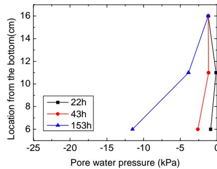
Fig.3 Isochronous curves of the PWP under 30 kPa vacuum pressure
