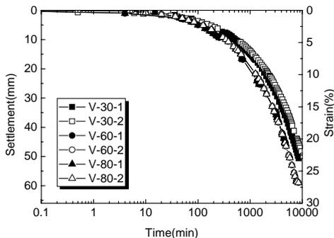
Fig.2. Comparison of settlement versus time with different magnitudes of vacuum pressures
