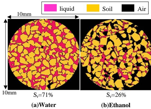
Figure 5 Threshold image after absorption
