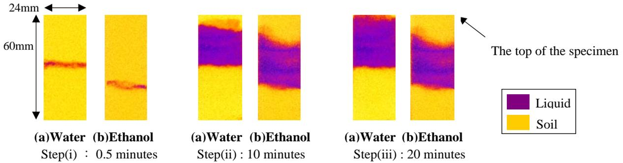
Figure 4 The subtraction diorama images on the absorption process in the sand specimen
