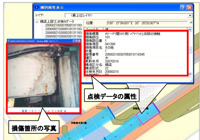
Fig. 1 Display of maintenance data and damage photograph.
