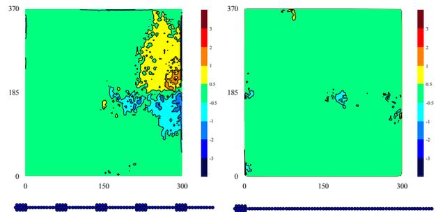
Fig.6 Vertical displacement field for different geogrid shape
