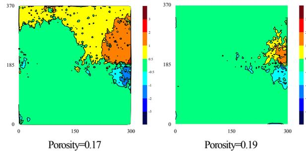
Fig.5 Vertical displacement field for different porosity
