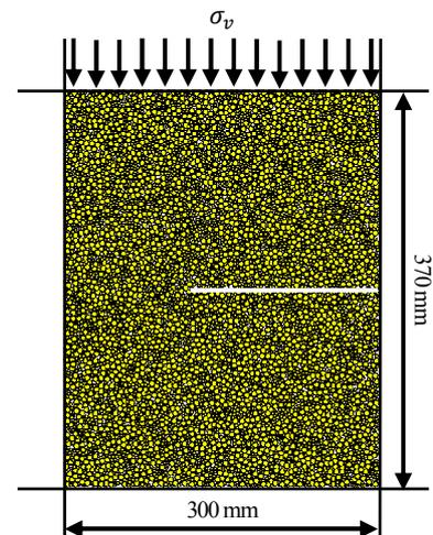
Fig.1. DEM model of pullout test
