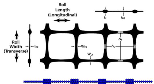
Fig.2. General dimensions and DEM model of geogrid
