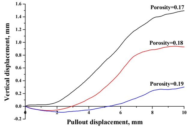
Fig.4 Vertical displacement of top wall for different porosities
