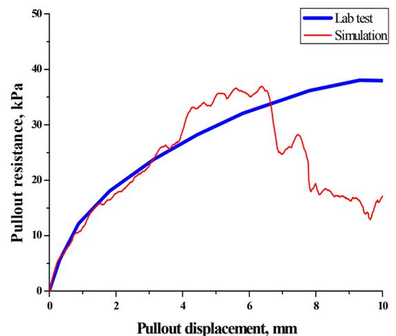
Fig.3 Pullout resistance as a function of displacement
