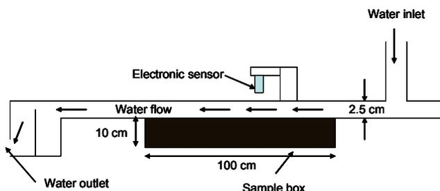
Figure 1. Experimental apparatus profile view
