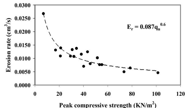
Figure 5. Correlation of peak compressive strengths and erosion rates
