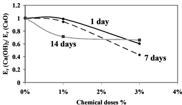
Figure 4. Comparison between the erosion rates for every dose of the volcanic ash sandy soil with both kinds of the chemical additives (the calcium hydroxide and the calcium oxide)
