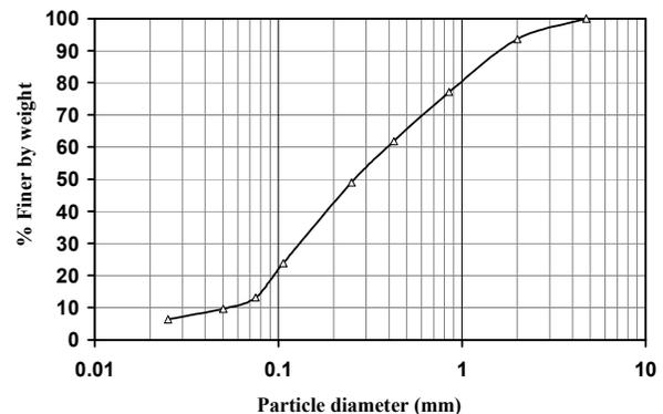
Figure 2. Grain size distribution curve for Shirasu soil specimen
