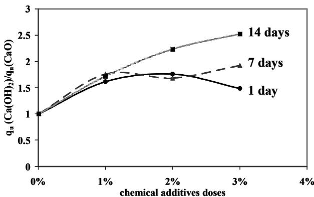
Figure 3. Comparison between the peak compressive strength for every dose of Shirasu soil with both kinds of the chemical additives (the calcium oxide and the calcium hydroxide)
