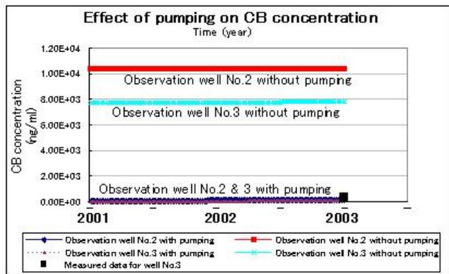
Fig. 3. Effect of pumping on CB concentration.
