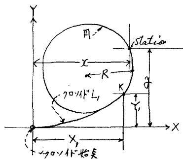
$$x = X_1 + R \left\{ G \sin \left( \frac{1}{2} \cdot \frac{L_1}{R} \right) + \sin \left( \frac{1}{2} \cdot \frac{L_1}{R} + \frac{\text{station} \sim K \text{墓間円弧長}}{R} \right) \right\} \dots \quad (4.1)$$
