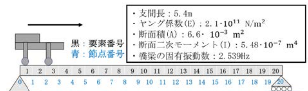
Fig.1 Beam model for simulation with mechanical properties.
