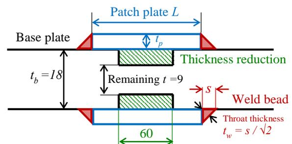
Fig. 1 Shape and dimension of specimen (mm)
