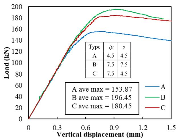
(a) Load and vertical displacement of A, B, C
