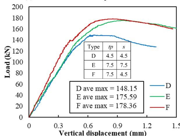
(b) Load and vertical displacement of D, E, F
