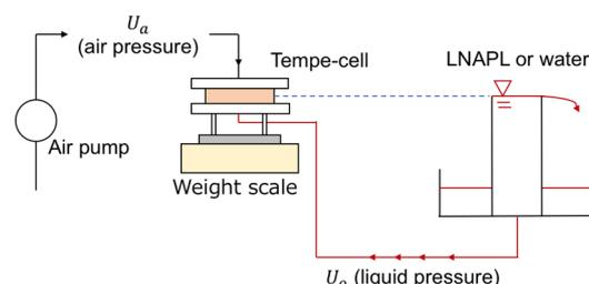
Figure 1. Schematic diagram of tempe cell test system
