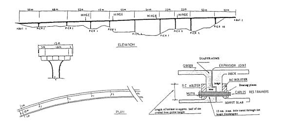
Fig. 1 Geometrical details of the Interstate-5/Route 14 Interchange. Separation and Overhead.
