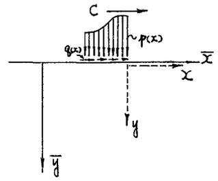
$$\left. \begin{aligned} \bar{\sigma}_x &= \lambda(\bar{u}_x + \bar{v}_y) + 2\mu\bar{u}_x \\ \bar{\sigma}_y &= \lambda(\bar{u}_x + \bar{v}_y) + 2\mu\bar{v}_x \\ \bar{\tau}_{xy} &= \mu(\bar{v}_x + \bar{u}_y) \end{aligned} \right\} \quad (1)$$
