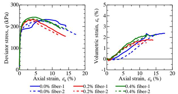
Fig.3 Consolidated drained triaxial extension test results performed under 300kPa confining pressure
