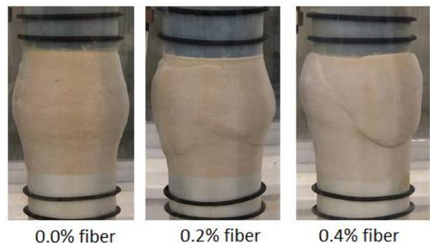
Fig.4 Failure modes of unreinforced and reinforced specimens under loading condition ( $p'_{\sigma}=200\text{kPa}$ )
