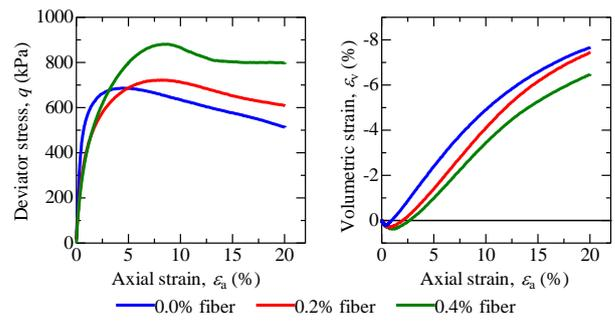
Fig.2 Consolidated drained triaxial compression test results performed under 200kPa confining pressure
