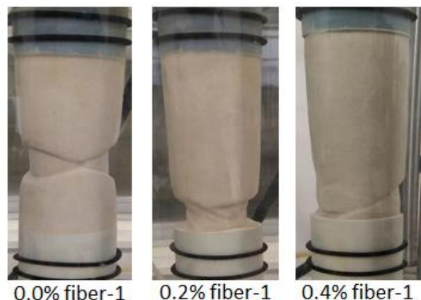
Fig.5 Failure modes of unreinforced and reinforced specimens under unloading condition ( $p'_{\sigma}=300\text{kPa}$ )
