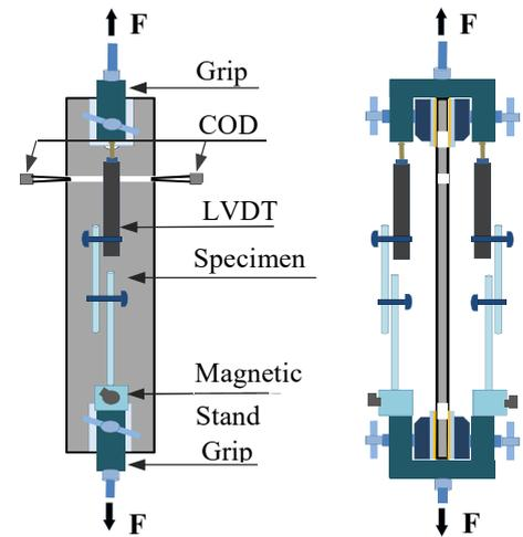
Fig 3 Test setup of pull-out test
