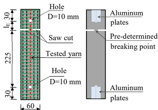
**Fig 2** Specimen used for pull-out test
