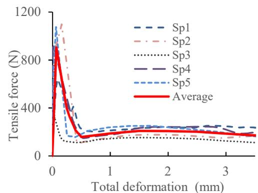
Fig 5 Tensile force - Total deformation relationship
