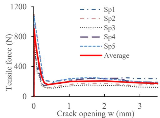
Fig 4 Tensile force - Crack opening relationship
