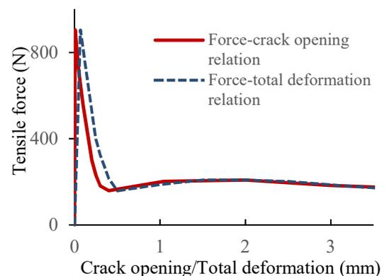
Fig 6 Comparison between Force-Crack opening relationship and Force-Total deformation relationship
