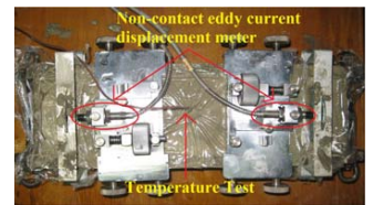
Fig.2 Non-contact shrinkage measuring instrument
