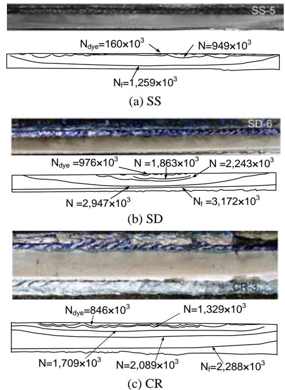
Fig. 3 Fractured surfaces
