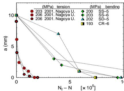
Fig. 5 crack depth and remained life
