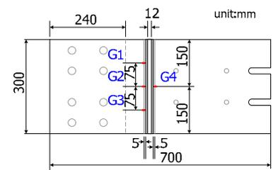
Fig.2 Strain gages location
