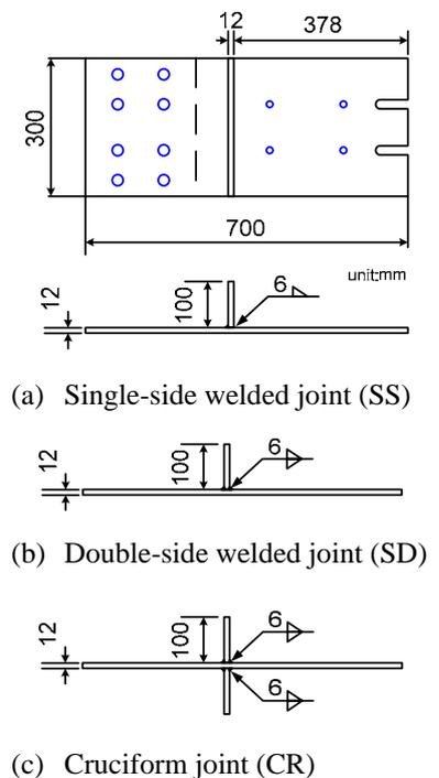
Fig.1 Fatigue test specimens
