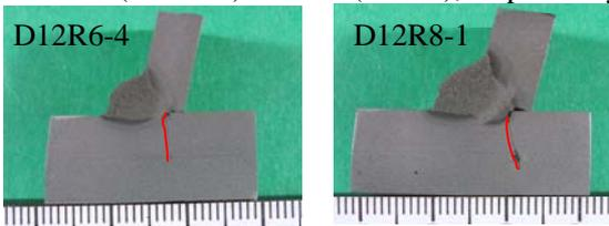
Photo 1 Macro-sections of weld root cracks
