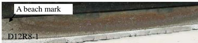
Photo 2 Beach marks left on a portion of main plate of a specimen
