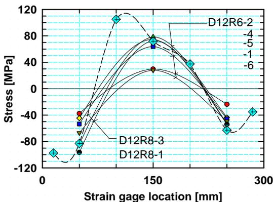
Fig. 6 Estimated residual stresses in weld root region
