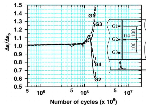
Fig.4 A pattern of variation in strain ranges for D12R6-1 specimen
