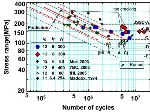
Fig.7 Comparison of test data and prediction
