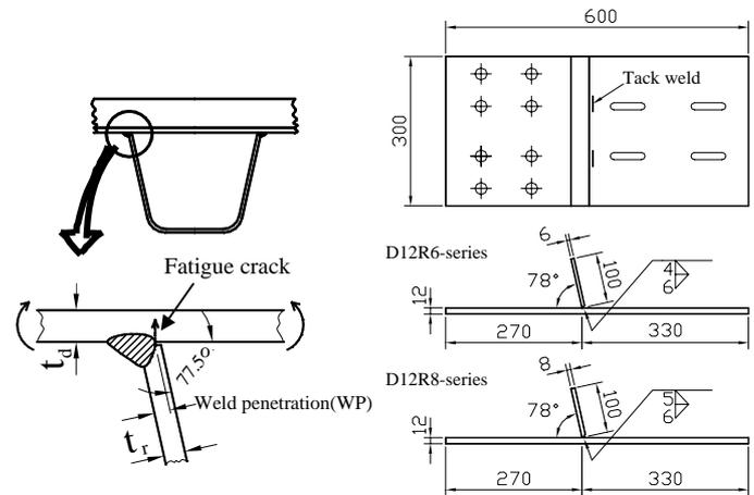
Fig.1 Fatigue crack in deck plate
