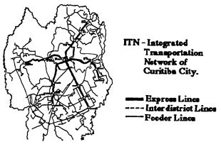
In 1974, an Integrated Transportation Network - ITN was introduced, constituted by 5 Express Lines running by 5 structural corridors in North, South, East and West directions integrated with Interdistrict and Feeder Lines.
