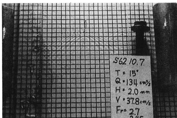
Fig.2 Surface waves in a laboratory shallow water channel. \alpha \approx 45.5^\circ , F_r = 2.7 , U = 0.38 \text{ m/s} , h = 0.002 \text{ m} .
