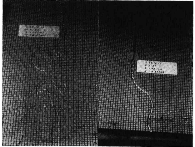
Fig.2 A meandering stream on the smooth Plexiglas surface. Slope length L \approx 72 cm, Surface slope \alpha = 15^\circ , Discharge Q = 8.5 cm 3 /s.
