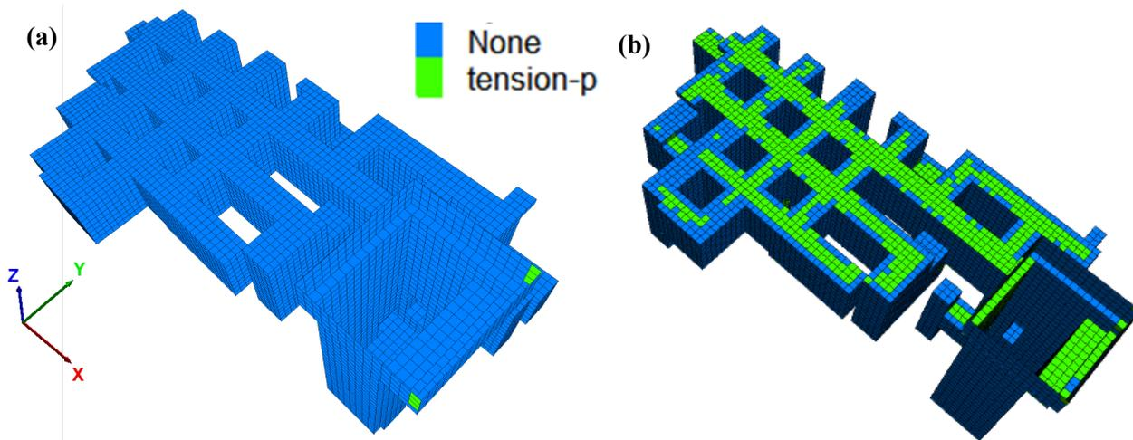
**Figure 5.** The excavated section showing yield zones (a) static (b) dynamic
