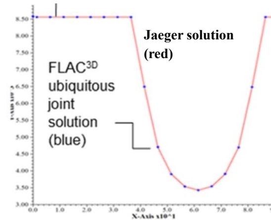
**Figure 2** showing the rock strength variation against the specified dip angle modified from (Sainsbury & Sainsbury, 2017).
