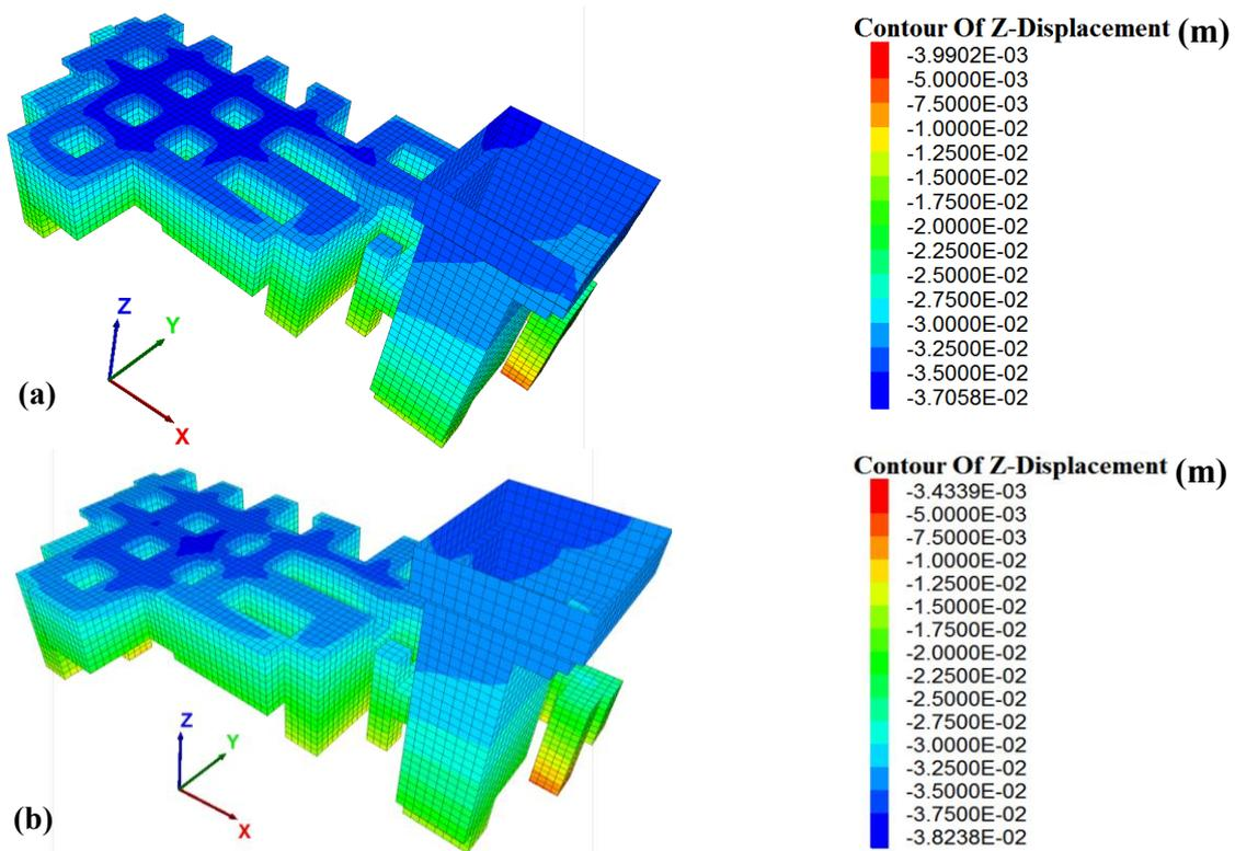
Figure 4. Displacement contours. (a) No joint, (b) with joint
