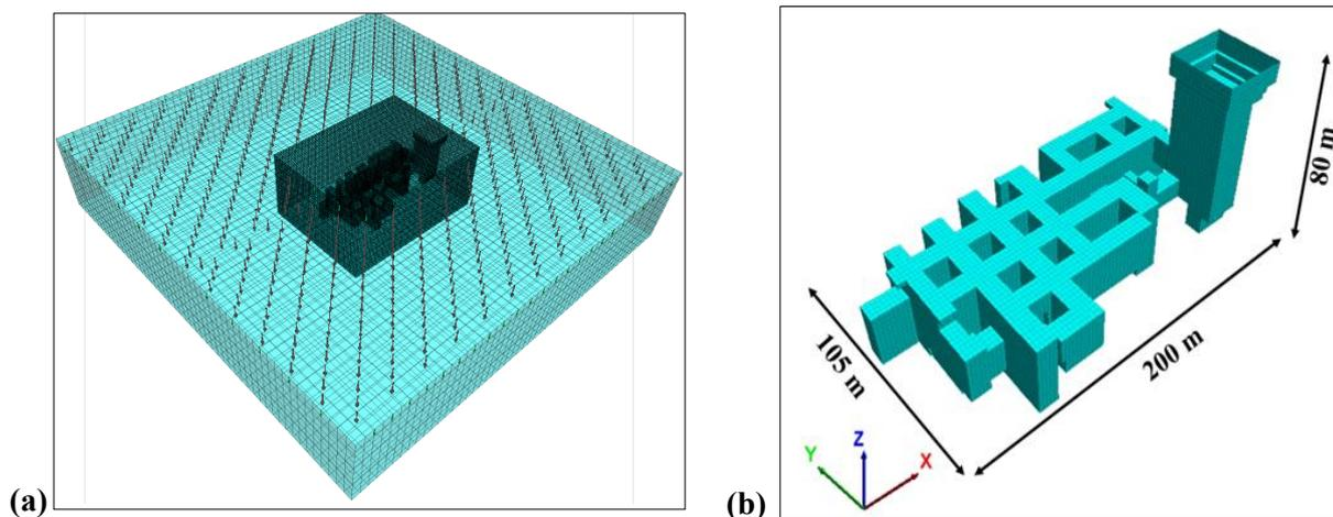
**Figure 3.** (a) 3D Model setup of Oya underground quarry; (b) excavated regio
