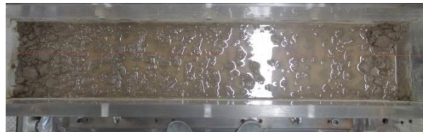
(b) 不飽和液状化 ( a_f = 600 \text{ Gal} , S_{rf}=81.7\% )
