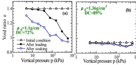
Fig. 2.  $e-p$  Relation of DL clay at  $S_r=20\%$
