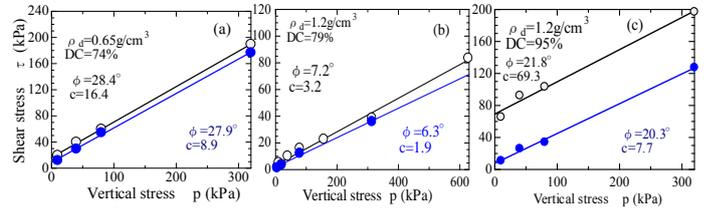
Fig. 6.  $\tau-p$  Relations (a) Kanto loam, (b) DL clay and (c) Kaolin clay
