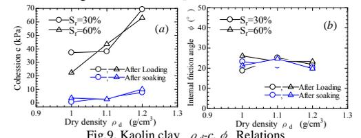
Fig. 9. Kaolin clay  $\rho_d, c, \phi$  Relations
