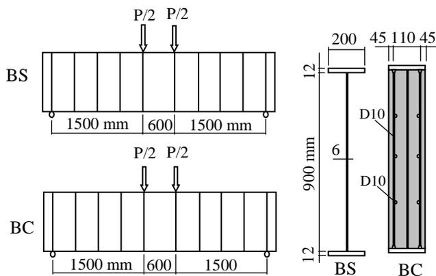
Fig. 6: Models for bending tests
