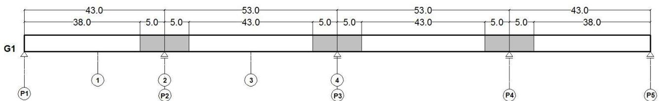
Fig. 1: Longitudinal view of Concrete filled I-Girder (CFIG) bridge (unit: m)
