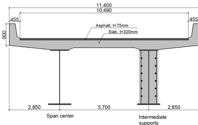
Fig. 2: Cross section of Concrete filled I-Girder (CFIG) bridge (unit: mm)
