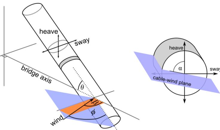
Figure 2: Definition of the geometric angles.
