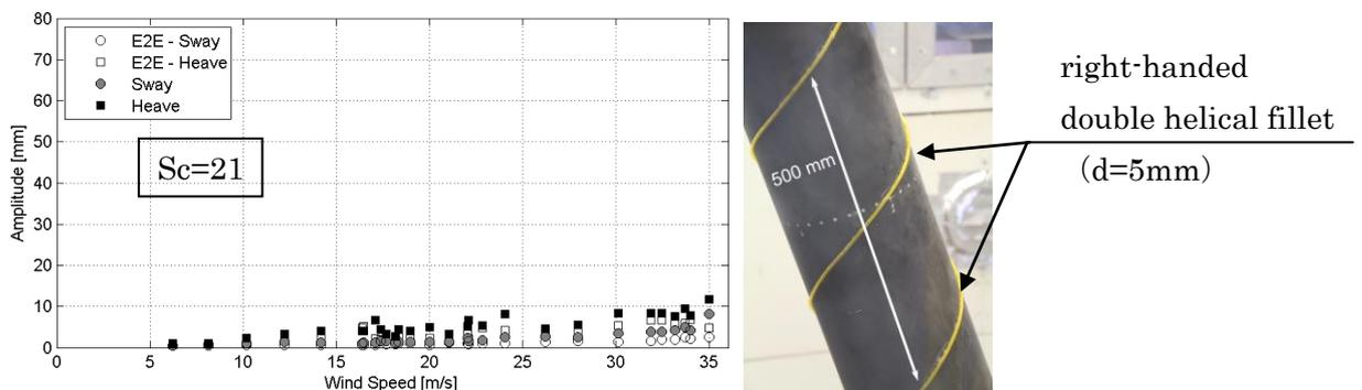
Figure 4: Test Result of the cable with helical fillet.
