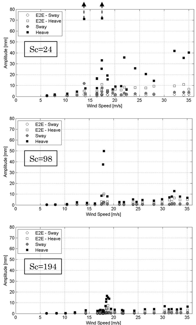
Figure 3: Test Results of the smooth cable.
