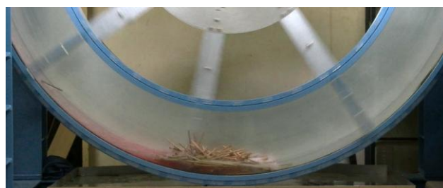
(c) 流木塊固化状態 ( h=70 mm, v=4.0 m/s, l=180 mm, n=300 )
