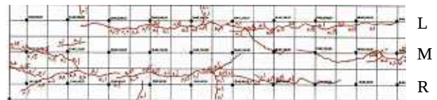
Fig. 5 Corrosion crack in concrete cover B-LM-0-20
